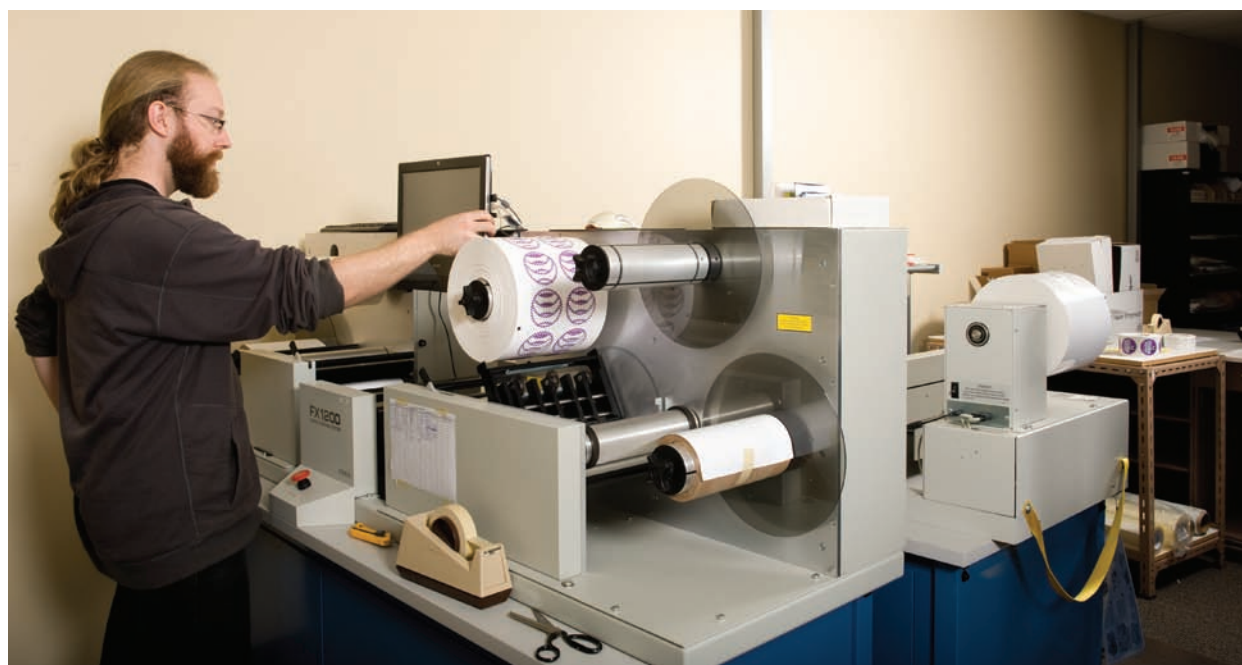
Sticky Business press operator Mike Reid preps the Prima Technology FX1200 Digital Finishing system comprising a die-cutter, laminator, weeder and finisher.
