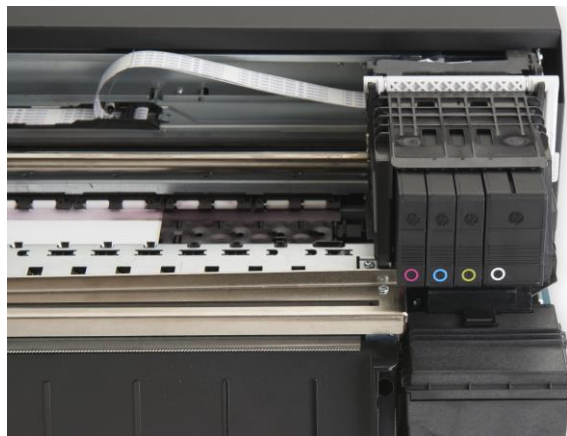
Separate ink tanks on LX2000 Color Label Printer
